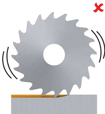
1 - 2 teeth in material Not enough teeth = risk of vibration
